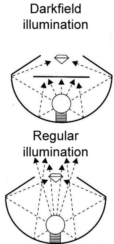
Figure 10. Darkfield and transmitted illumination.
