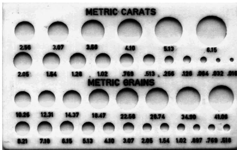
Figure 4. Hole gauge for estimating diamond and pearl weights.
