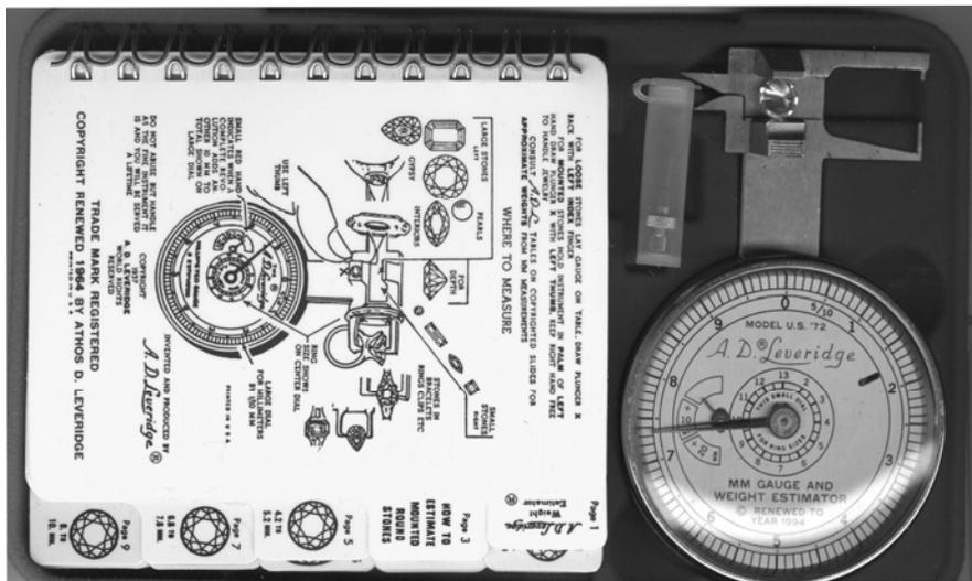
Figure 7. The Leverage gauge. Used to estimate diamond weight very accurately, including in mounted jewelry. Stone diameter in this picture is 7.39 mm! The small cylinder case contains a probe for finding the height/depth in mounted stones.
