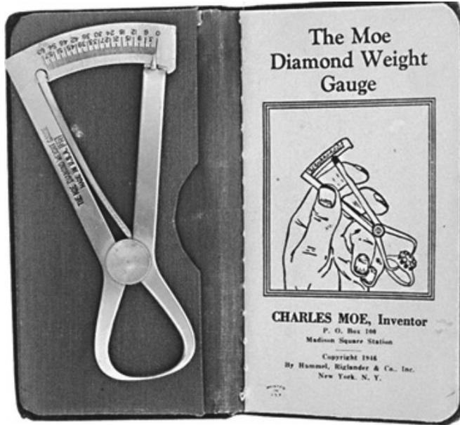
Figure 5. The Moe Gauge. It is used for diamond weight estimation.
