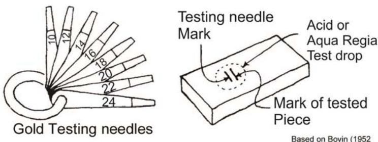
**Figure 1. Gold testing using acid.**
