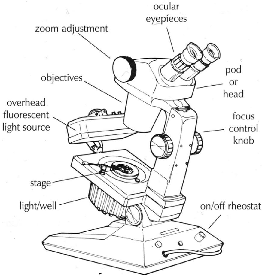
Figure 9. Diamond microscope.
