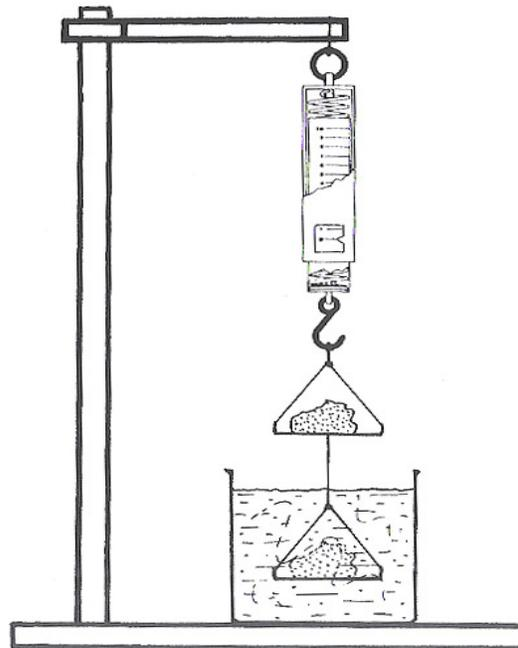
Figure 5. Weighing a mineral in air or water.
