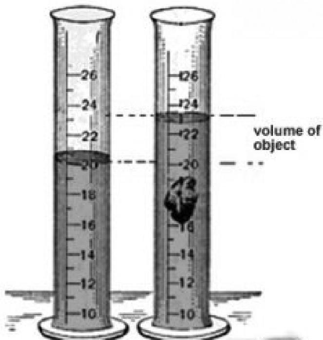
Figure 9. A volume change. The mineral is suspended on a piece of string.
