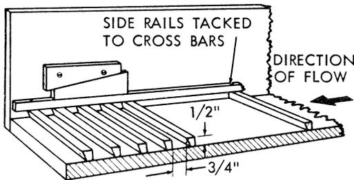
FIGURE 17. – Wooden riffle suitable for use in a sampling sluice.
