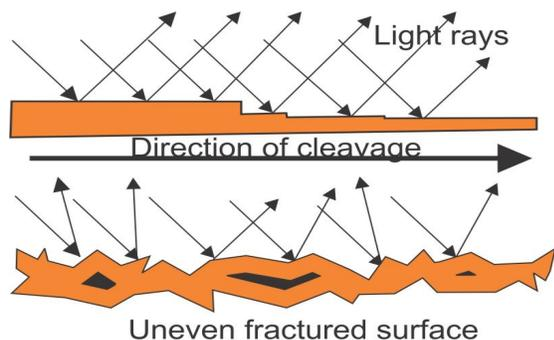
Figure 3. The flat or stepped surfaces of cleavage reflect light all in the same direction, like a mirror. A fractured uneven surface reflects light in all directions. Cleavage shows a strong flash of light when the specimen moves.
