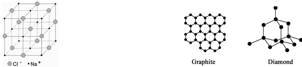
**Figure 1.** Shown above are the crystal structure (magnified and expanded) of the minerals, Halite (NaCl) and of two carbon minerals, graphite and diamond. The lines between atoms represent chemical bonds. The structure of minerals and their bonding make a lot of the difference in the minerals' properties, for example hardness.
