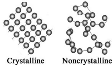
**Figure 2.** Crystalline and amorphous solids. Both are held by chemical bonds, but crystalline solids have an ordered structure that fills space in 3 dimensions. You can predict where the next atom can be found in the structure.
